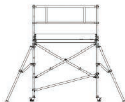
BASE UNIT & GUARD RAIL PACK Platform Height: 1.9m Reach Height: 3.9m
