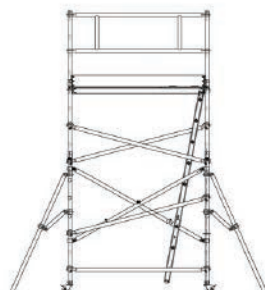
BASE UNIT & GUARD RAIL PACK WITH 1 x 1M EXTENSION Platform Height: 2.9m Reach Height: 4.9m
